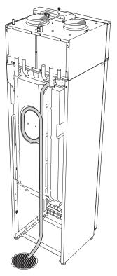
The condensation hose from FLM S45 has to be shaped into a water seal. On the rear of S1255 there is a groove in the insulation for the condensation hose; other compatible heat pumps do not have this groove.
