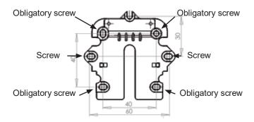
Hold up the wall frame against the wall and mark off the holes for fastening the frame. Drilling of holes, hole size and suitable screws for fixing the panel all depend on the wall material.
