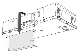
2. Unscrew all the screws holding the bottom panel.
