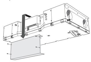
2. Unscrew all the screws holding the bottom panel.
