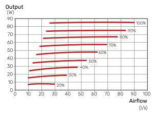
$^{1}\!\text{The diagram}$  shows the power consumption per fan.
