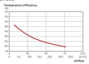
Outdoor air: 5 °C Exhaust air 25 °C RH exhaust air: <27.7 %
