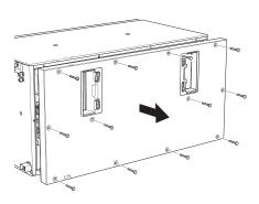
4. Unscrew both of the screws at the top and lift off the top panel.
