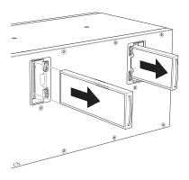
3. Unscrew the screws as illustrated and pull out the front panel.
