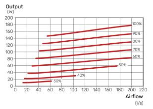
$^{1}\!\text{The diagram}$  shows the power consumption per fan.
