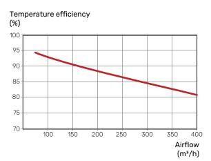
Outdoor air: 5 °C Exhaust air 25 °C RH exhaust air: <27.7 %
